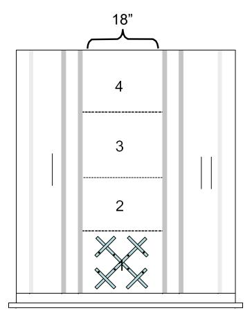
Test these hoods with an 18" horizontal opening. Try to make the opening toward the middle. Take a representative sample with the VelGrid staying at 3" inches from the left or right sides. Visual smoke testing should be conducted in the middle, 6" from the plane of the sash.
